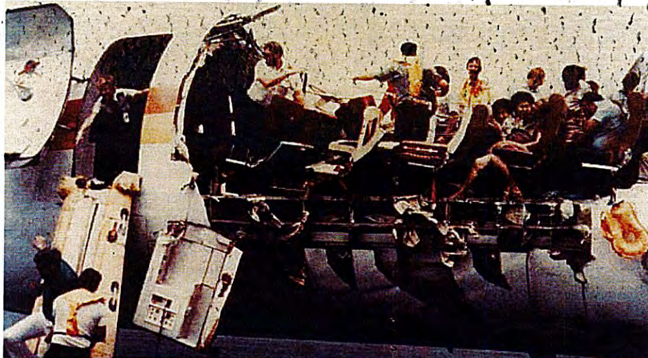
4-28-1988 After 89,090 flight cycles on a 737-200, metal fatigue lets the top go in flight.
